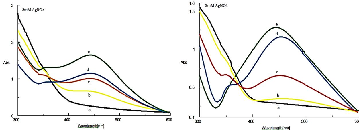
Fig. 4. Effect of ratio extract:AgNO<sub>3</sub> (3mM, 5mM), on production of AgNPs a. 5:1, b. 4:2, c. 3:3, d. 2:4, e.1:5
