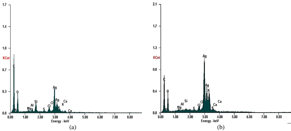
Fig. 10. EDX spectra of the AgNPs obtained using 3 mM AgNO<sub>3</sub> (a) and mM AgNO<sub>3</sub> (b)
