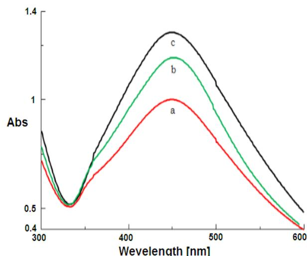
Fig. 3. Effect of different concentrations of AgNO<sub>3</sub> on the production of AgNPs a. 3 mM, b. 5 mM, c. 10 mM
