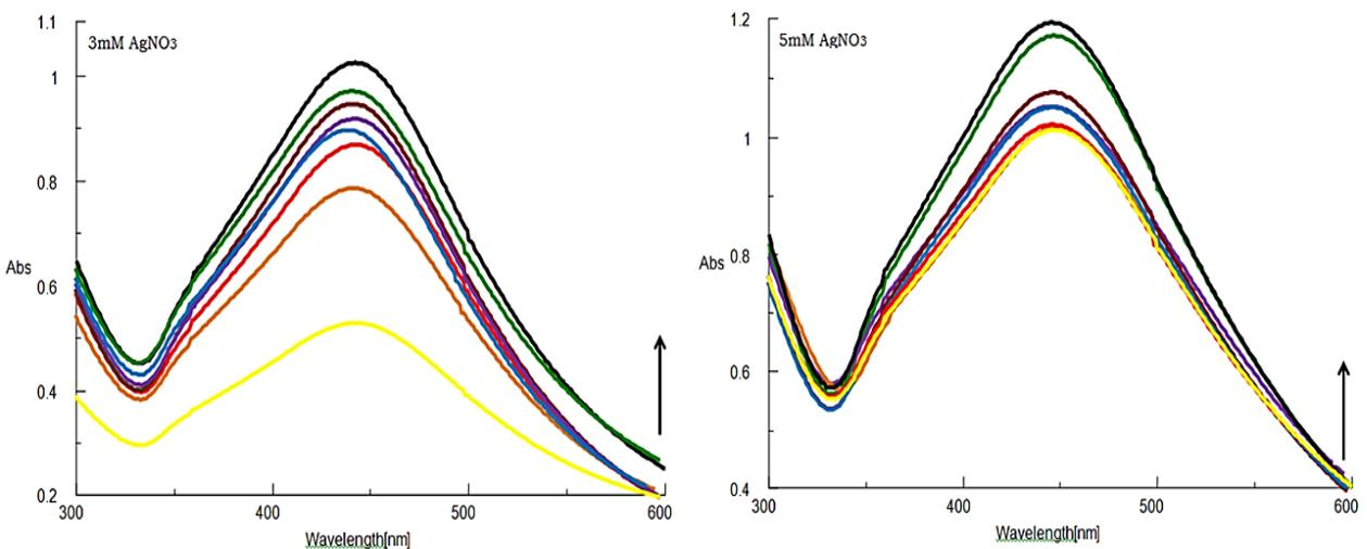
Fig. 7. Effect of stirring time on production of AgNPs: 15', 30', 45', 60', 90', 120', 180', 240'
