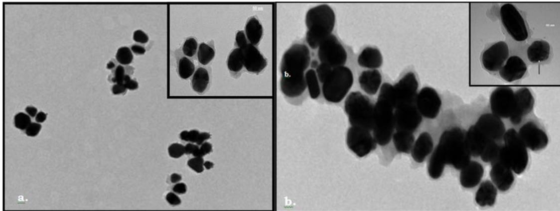
Fig. 9. TEM images of AgNPs using a. 3 mM AgNO<sub>3</sub> and b. 5 mM AgNO<sub>3</sub>
