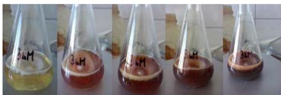
Fig. 1. Visual observation of synthesis process of AgNPs, in time
