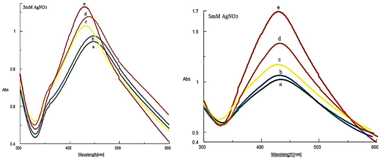
Fig. 6. Effect of temperature on production of AgNPs: a. 25 °C, b. 35 °C, c. 50 °C, d. 70 °C, e. 90 °C
