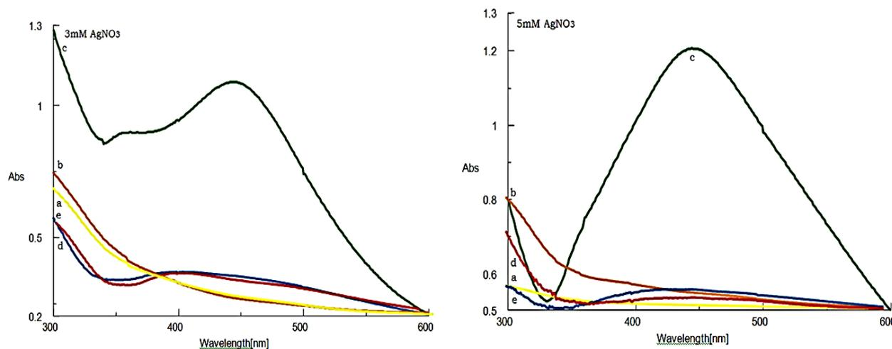
Fig. 5. Effect of pH on production of AgNPs: a. pH 2, b. pH 4, c. pH 6, d. pH 8, e. pH 10
