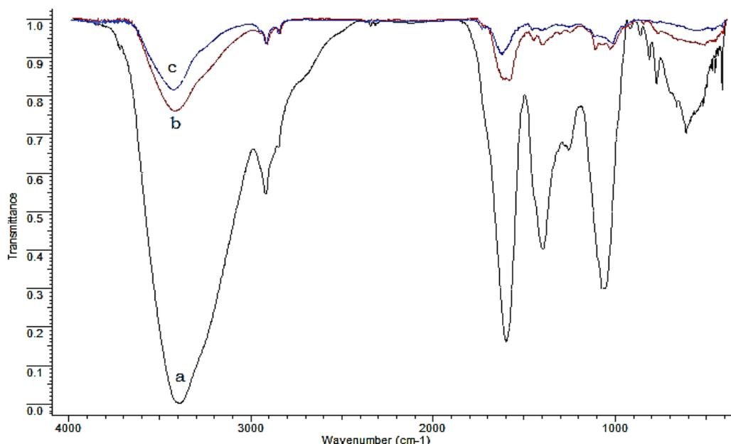
**Fig. 8.** FTIR spectra of a. extract and AgNPs obtained using b. 3 mM AgNO<sub>3</sub> and c. 5 mM AgNO<sub>3</sub>
