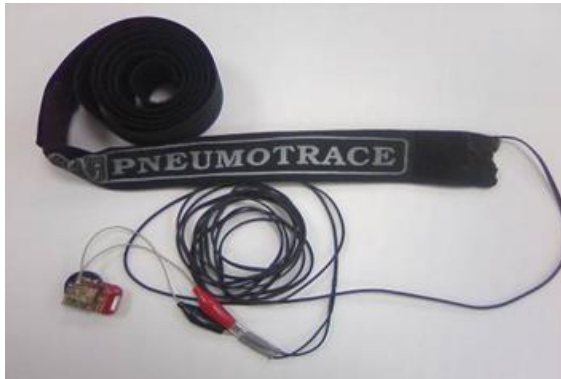
Figure 17c. Device for telemonitoring the respiratory system
