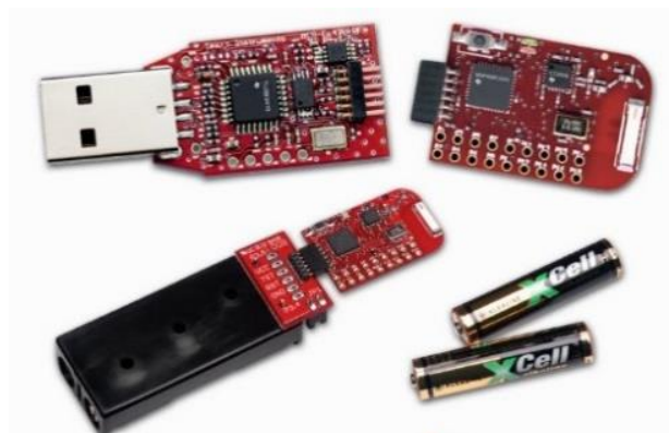
Figure 17b. Device for telemonitoring the heart rate and blood-oxygen saturation (microcontroller and wireless transceiver)
