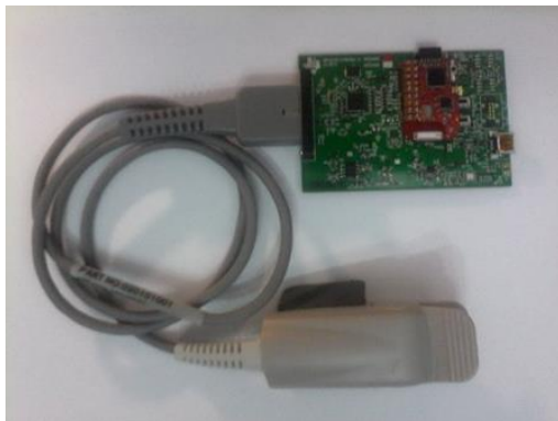
Figure 17a. eZ430-RF2500 wireless development kit
